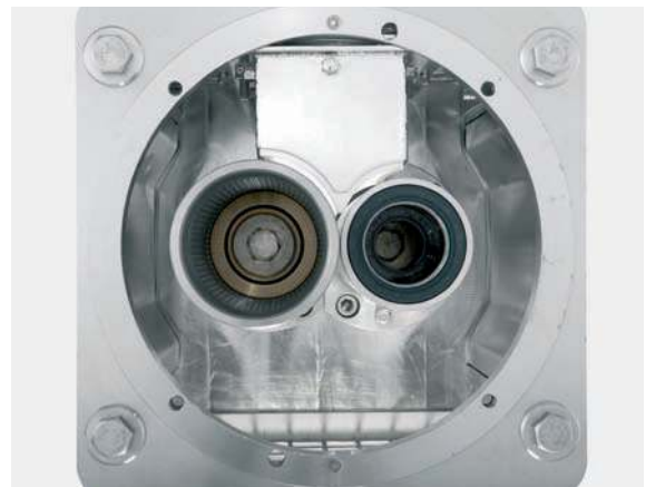
The ratio between the bore length and bore diameter, and the ratio between the circumferential speeds determine the degree of compaction, and thus the properties of the finished granule.
