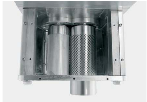
The pressure cylinder forces the material through the bores of the granulating cylinder.
